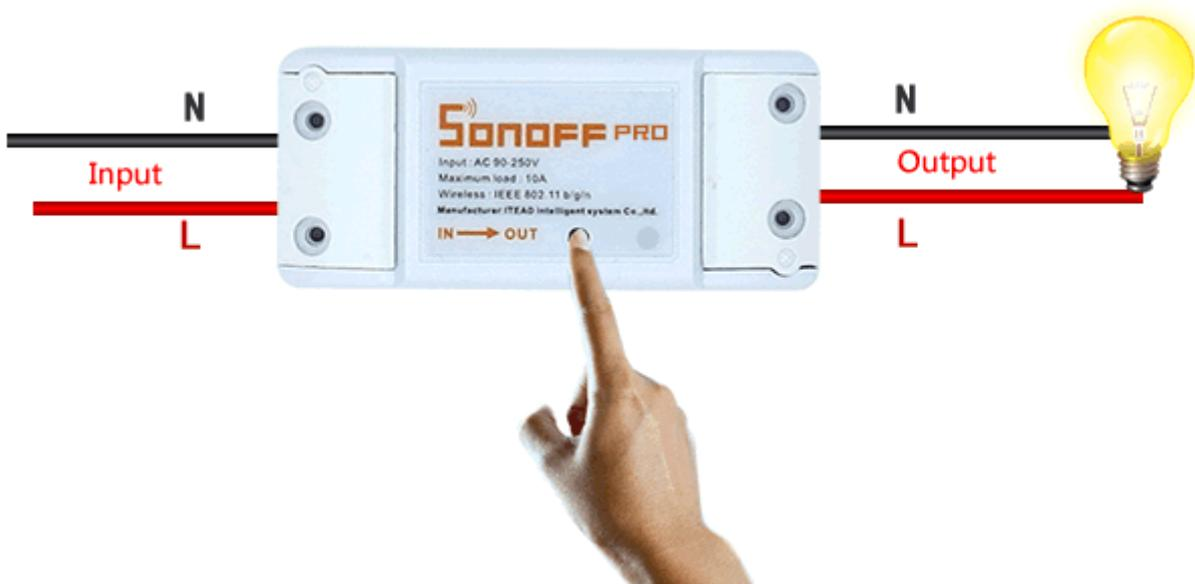
Fast press the black button on Sonoff RF for three times, the red LED is on for 3s, that means the RF controller code has been cleaned. If you failed to pair, please try to clean first.
